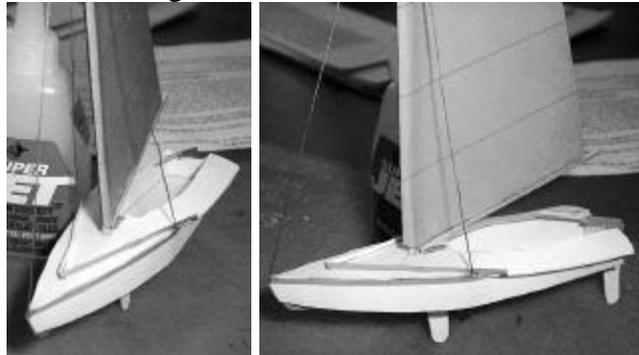
17. Fold the jib sail over on itself with the blue facing out. Open back up and put glue on the inside of the sail. Fold the sail back together over the forstay ( string on the front of the boat.) and press together.
